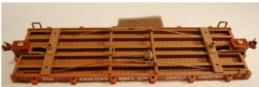
The old frame has the truck bolster below the side sill. This article addresses the old frame.
