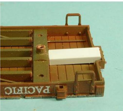
Cut a piece to fit between the bolster and the frame end.
