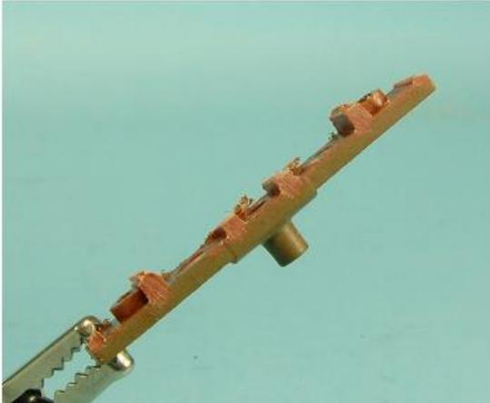
**Nip off the frame pieces from the bolster. The frame member has to be filed down level with the truss rod lug.**
