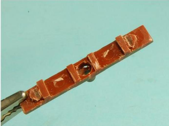
File grooves in the lugs to accommodate the truss rods. Use a hack saw blade and a file.
