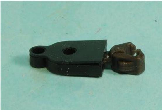
Accurail's standard HO coupler is the correct size for the modern narrow gauge era. The Accurail coupler doesn't have the hinky spring and the pencil neck of the other HO couplers.
