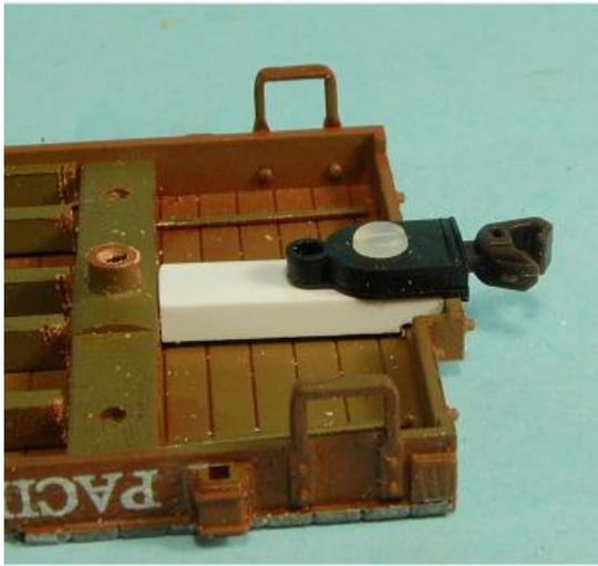
The lug on the coupler latches over the buffer block on the car. If the coupler doesn't quite fit file on the coupler block.
