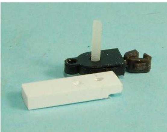
Drill and tap a #2-56 hole 5/32 from the end. Use a nylon screw 3/16 long to mount the coupler. Nylon screws are easier to cut and use.
