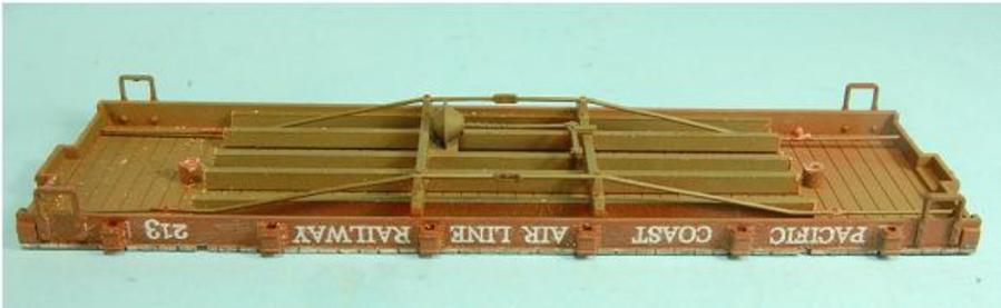
Glue the truss rods with a small drop of CA on the kingpost. Make sure the turnbuckles are vertical and centered.
