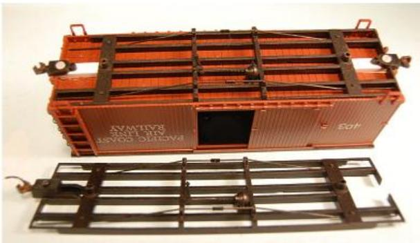
There are two version of Bachmann On30 cars. The late version have this underframe. The bolster is even with the side. There are replacement underframes available but the price has skyrocketed. All that is needed is a new coupler pad and new trucks.
